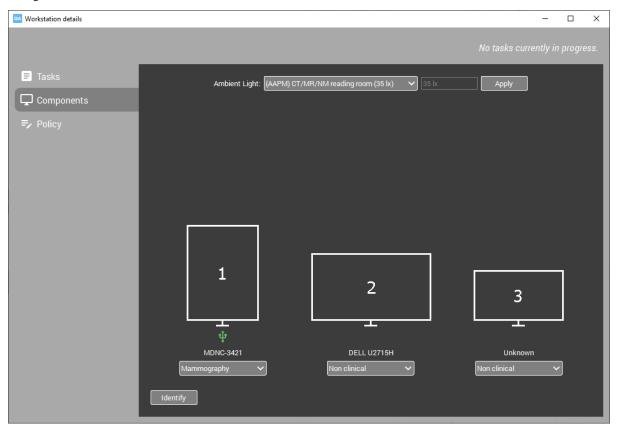
To verify the physical location positioning of the displays, click the **Identify** button. A display number indication will be temporarily shown on each display.
